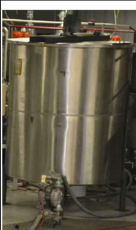
Figure 4. Exemplar AB Specialty batch tank with agitator and lid. (Credit: AB Specialty)
